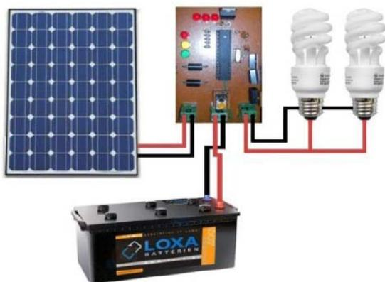
Figure 1C : Basic image of controller and battery wiring [18]
