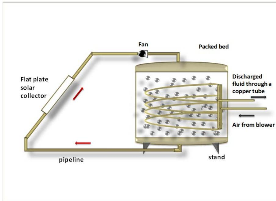
Figure 1.0 : Schematic of Storage systems for optimization
