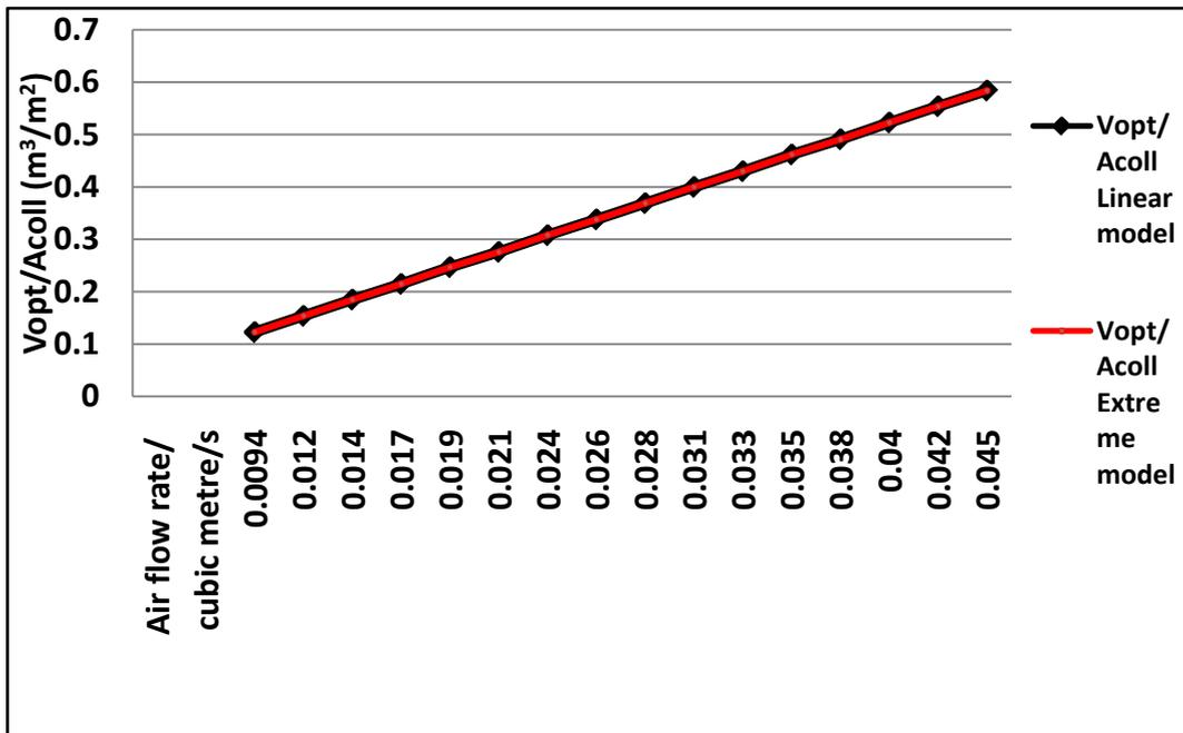
Figure 5.0 : Relationship between the optimum volume of packed bed storage system and the air flow rate obtained from the extreme and linear models
