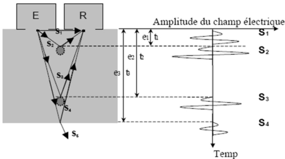
Picture 3 : Schematic diagram of the radar auscultation on a reinforced concrete slab
