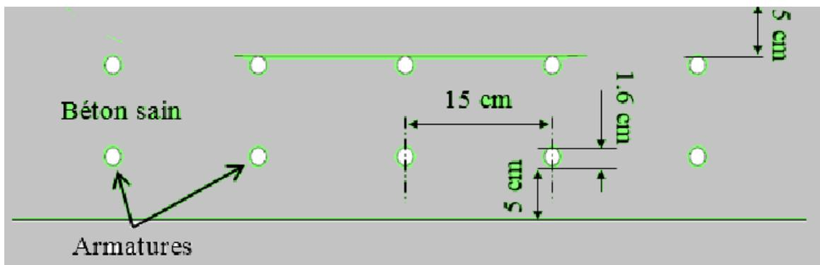
Picture 8 : Model of fissure in reinforced concrete
