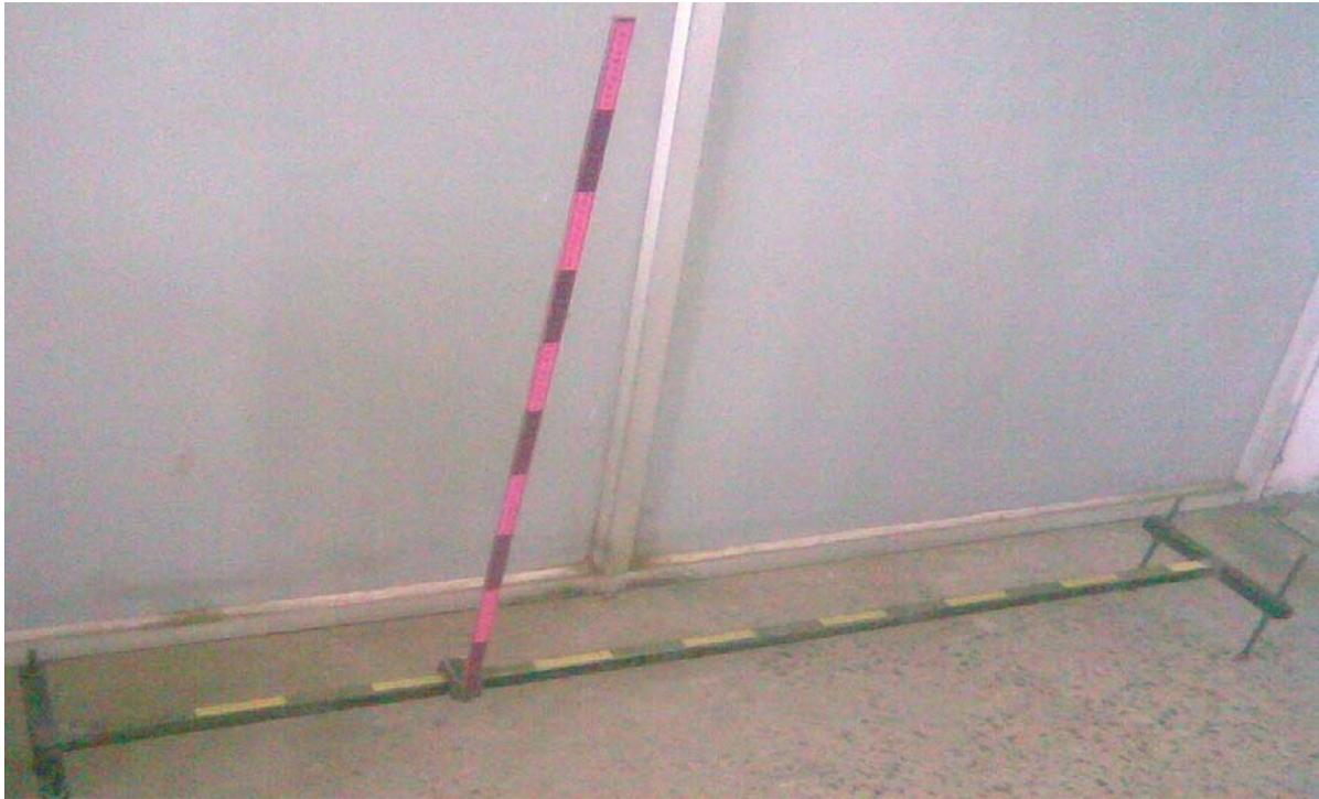
Figure 2 : Linear scales for measurement of parabolic profil
