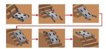
Figure 5.3: Simulation of staircase obstacle scenario
