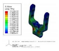
Figure 6.6: The stress of anti-vibration cantilever structure vs. the load of 100kg
