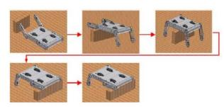
Figure 5.2: The simulation of obstacle crossing scenario
