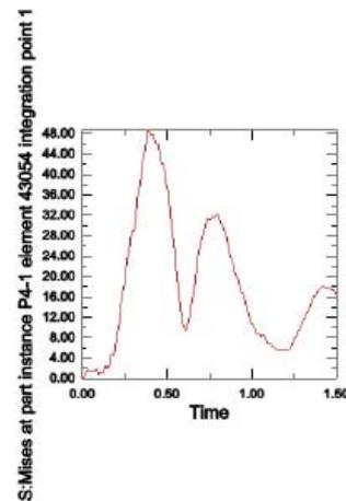
Figure 6.8 : The stress variation curve within 1.5 second interval at the location of main structure element 43054
