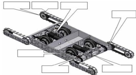
Figure 4.2 : Prototype design of vehicle with in-wheel motor (interior)
