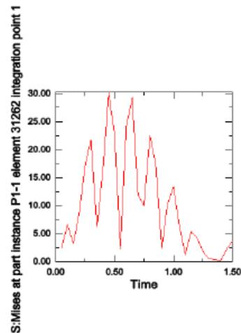
Figure 6.12 : The stress variation curve within 1.5 second interval at the location of in-wheel cantilever structure element 31262
