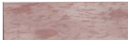
Fig. 1: Microscopic picture of Sample 1 after 70 days (groundnut emulsion as cutting fluid)
