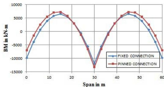
Fig. 10 : Comparison of BM variation in deck slab of two spans integral abutment bridge due to DL for pile head with fixed and pinned connection
