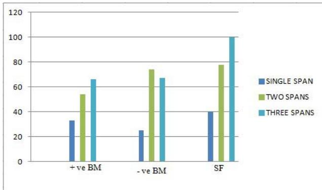
Fig. 21 : Comparison of percentage changes in all the parameters considered in exterior girder of single, two and three spans integral abutment bridge due to DL+ LL + temperature with respect to DL
