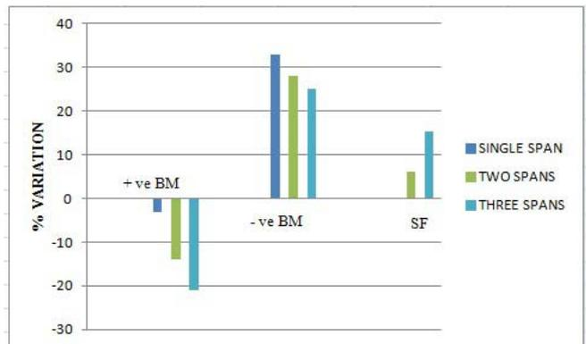
Fig. 19 : Comparison of percentage changes in all the parameters considered in exterior girder of single, two and three spans integral abutment bridge due to DL+ temperature with respect to DL
