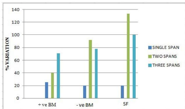
Fig. 22 : Comparison of percentage changes in all the parameters considered in central girder of single, two and three spans integral abutment bridge due to DL+ LL + temperature with respect to DL
