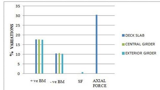
Fig. 9 : Comparison of percentage changes in all the parameters considered in deck slab, central girder and exterior girder in single span integral abutment bridge having pile head with pinned connection under DL with respect to single span bridge with fixed pile head
