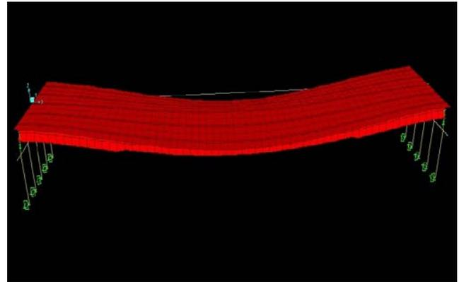
Fig. 4 : Deformed shape of the single span integral abutment bridge model for live load
