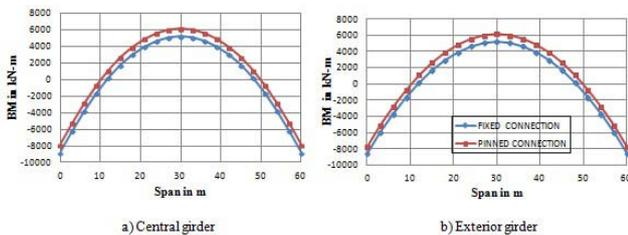
Fig. 7 : Comparison of BM variation in (a) central girder and (b) exterior girder due to DL for single span pile head with fixed and pinned connection
