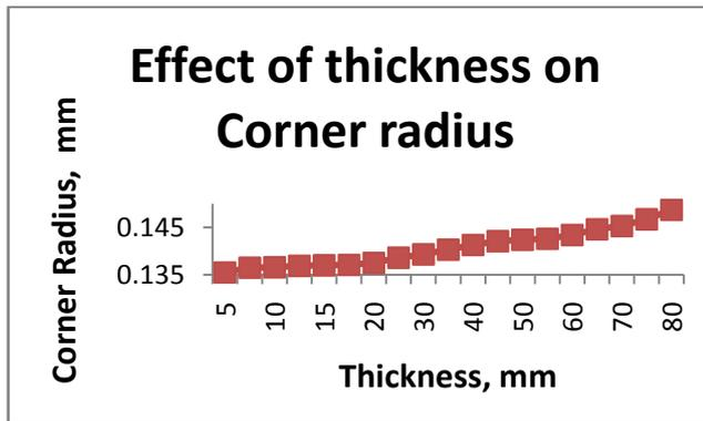
Figure 5 : Effect of workpiece thickness on corner radius
