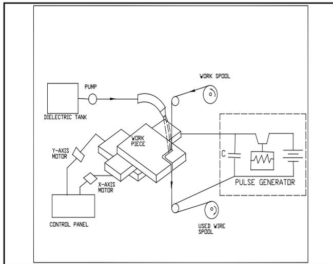
Figure1 : Wire electrical discharge machining Process
