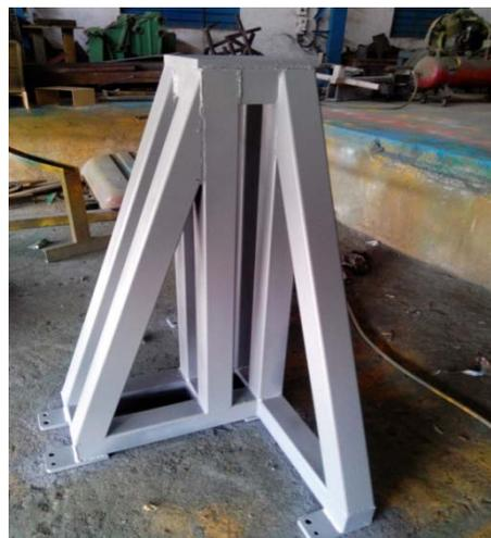
Figure 9 : Motor mounting
