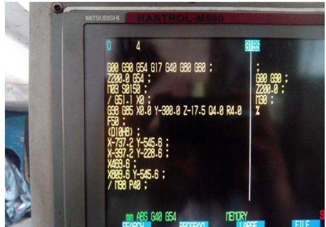
Figure 23 : G-code for Drilling
