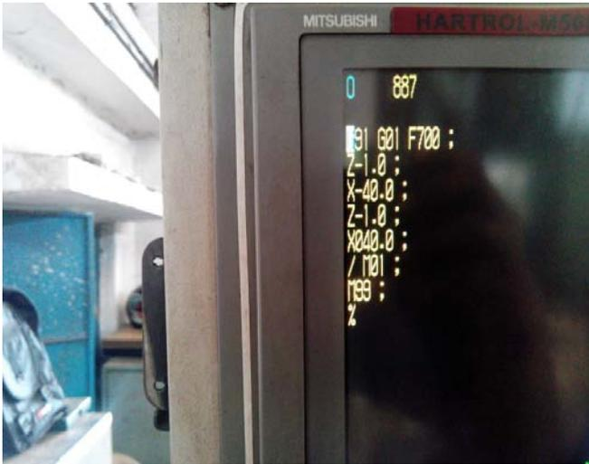
Figure 25 : G-code for Milling
