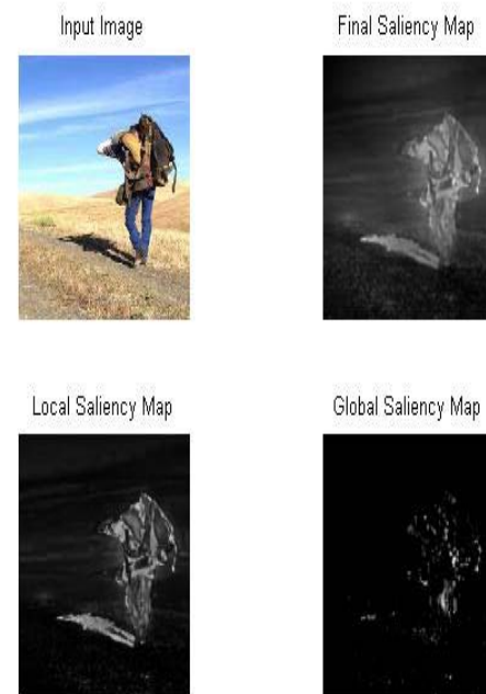
Fig. 5 : Local, Global and Final saliency map for a given image by using DWT
