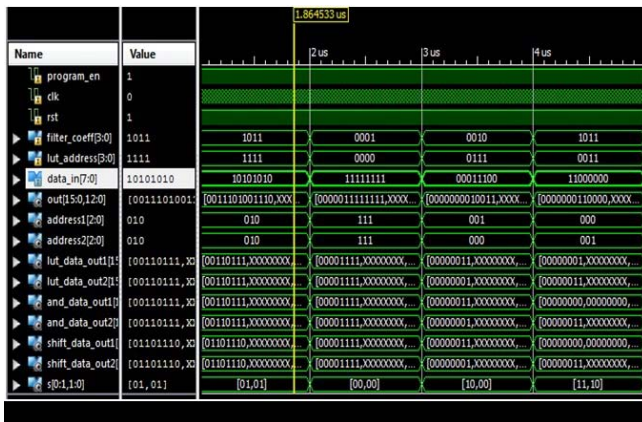
Fig. 7 : Simulation result of 16-bit LUT
