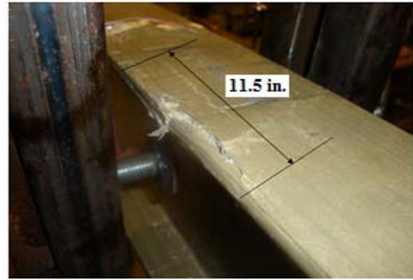
Fig. 4 : Top flange GFRP beam cracking in Experiment 1
