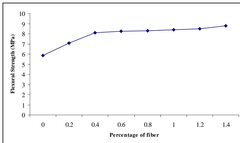
Figure 2: Variation of flexural strength
