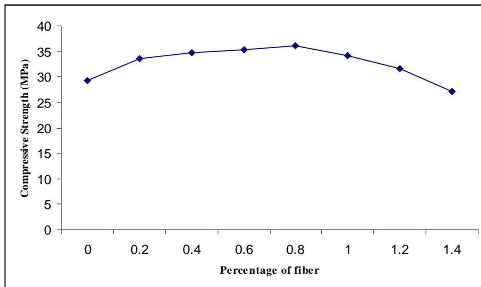
Figure 1: Variation of compressive strength of SIFF
