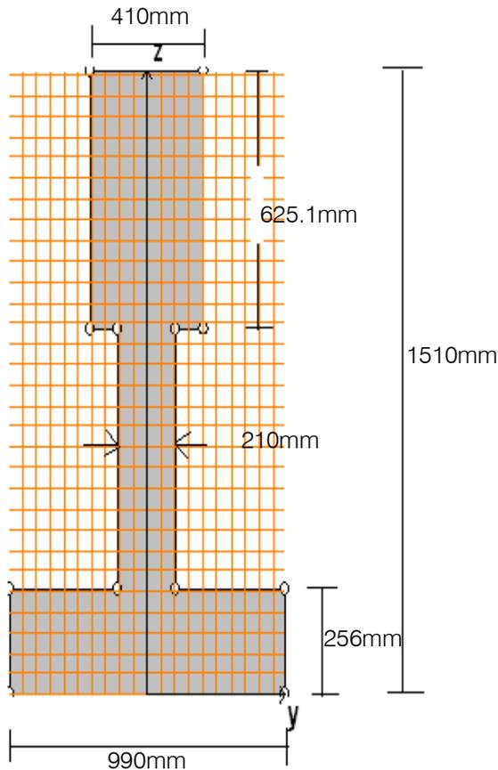
Figure 1 : Section of inverse-T girder
