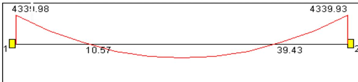
Fig 2 : Typical Inflection Point Diagram
