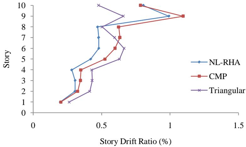
Figure 4.2 : Height-wise distribution of drift ratio for asymmetric model with 5% eccentricity
