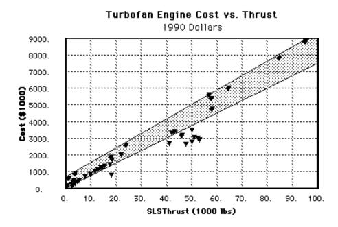
Figure 2 : Engine prices (\$1990) vs. SLS thrust (lbs)
