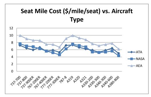
Figure 4 : SMC for ATA, NASA, and AEA methodologies
