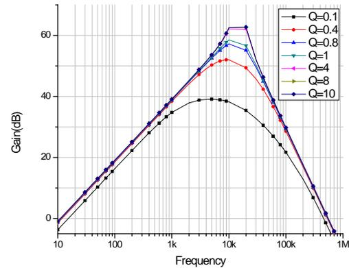
Figure 5 : Band-pass (BP) response for different values of Q
