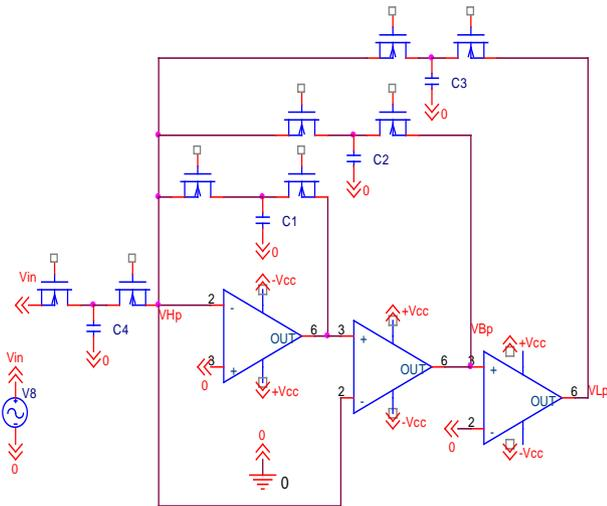
Figure 2. Proposed Circuit diagram for Electronically Tunable Third Order Switched-Capacitor filter
