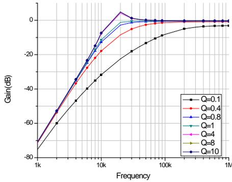
Figure 4 : High-pass (HP) responses for different values of Q
