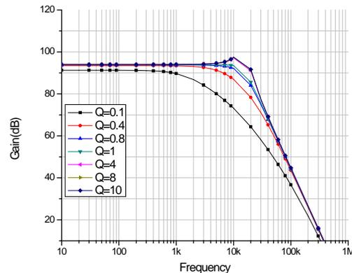
Figure 3 : Low-pass (LP) responses for different values of Q
