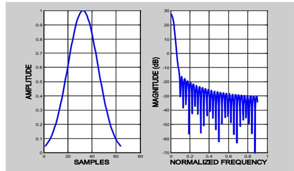
Figure 2.1 : The time and frequency description of a Gaussian Window with "α=2.5"
