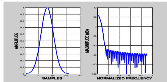
Figure 2.2 : The time and frequency description of a Gaussian Window with "α=3.5"
