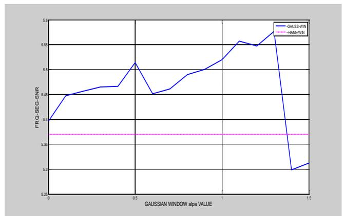
Fig. 2 (d) : Speech quality Objective Measures LLR and FSG-SNR Variation With "α", (CAR-NOISE of 0dB SNR)
