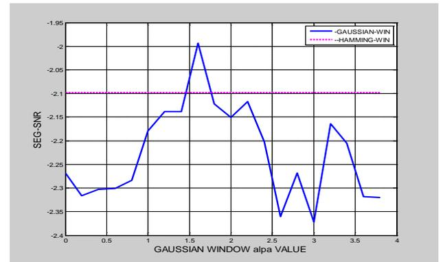
Fig. 2 (e) : Speech quality Objective Measures SEG-SNR and SNR Variation With “ $\alpha$ ”, (CAR-NOISE of 0dB SNR)
