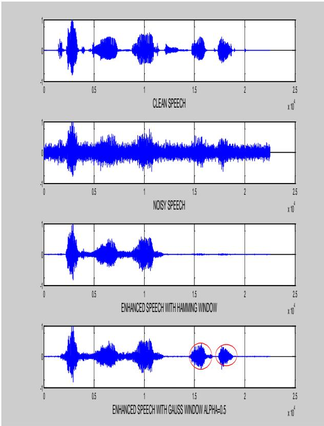
Fig. 2 (a) : Speech Signal Enhancement comparison ( $\alpha=0.5$ , CAR-NOISE of 0dB SNR)
