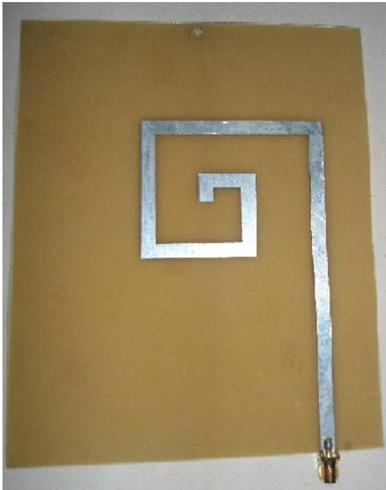
Figure 5 : Photograph of fabricated increased turns rectangular microstrip spiral antenna
