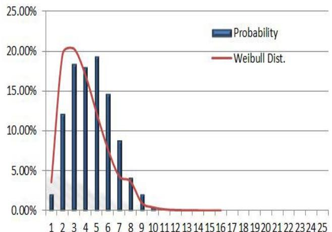
Figure 7.2 : Histogram for monthly mean speed with probability and weibull distribution of wind speed
