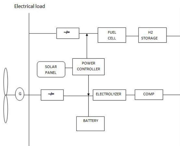
Figure 7.4 : Proposed power system consisting of wind, hydrogen and solar
