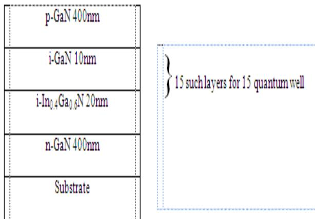
Figure 2 : Proposed model of MQWsolar cell
