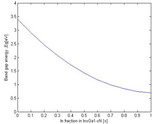
Figure 1 : Calculated band gap energy of semiconductor as a function of Indium fraction x
