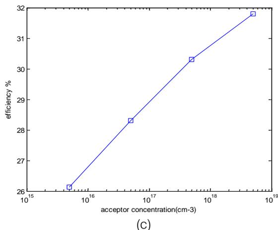
Figure 5 : Variation of (a)  $V_{oc}$  (b)  $J_{sc}$  and (c)  $\eta\%$  with Na when  $N_d=5 \times 10^{17} \text{ cm}^{-3}$
