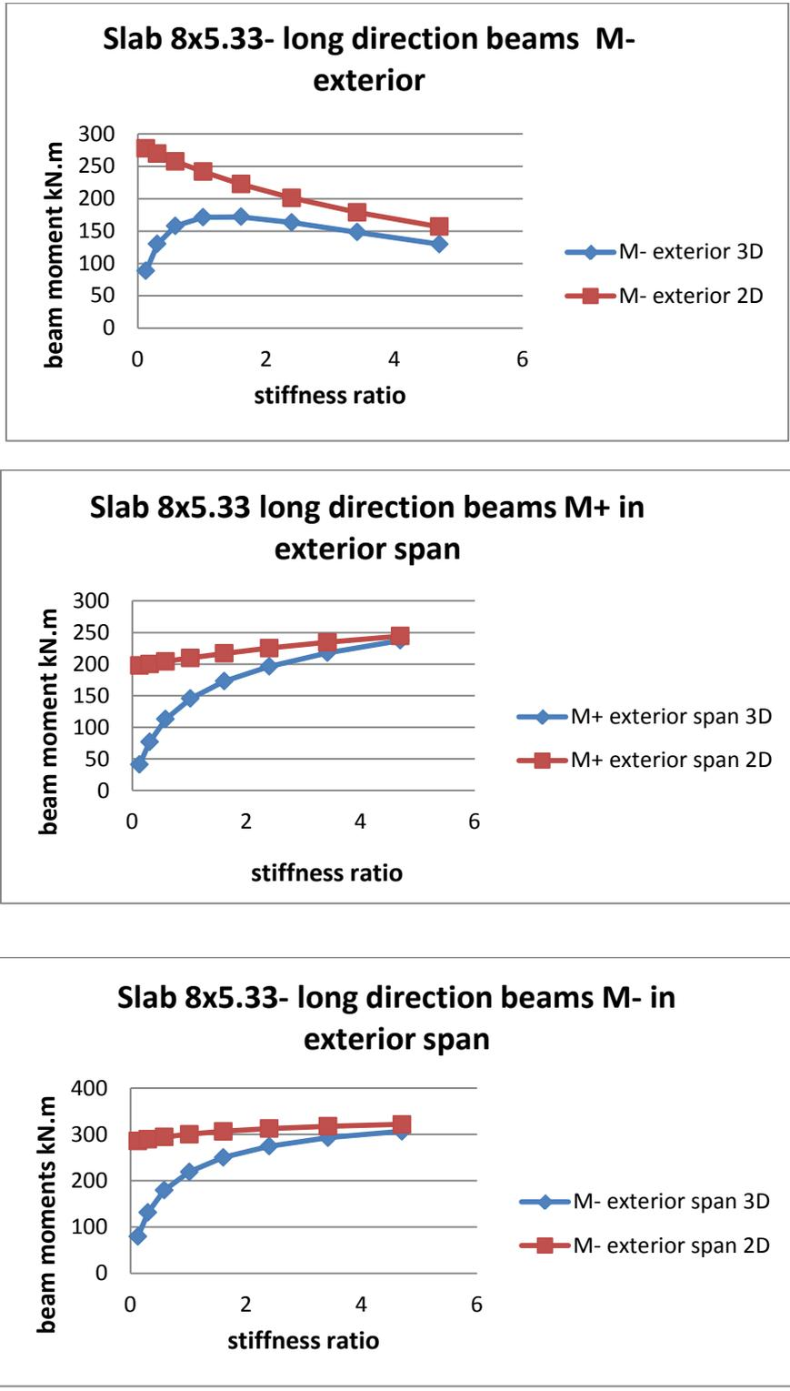
Figure 1 : Relation Between moments in beams determined by three and two dimensional analyses- F
