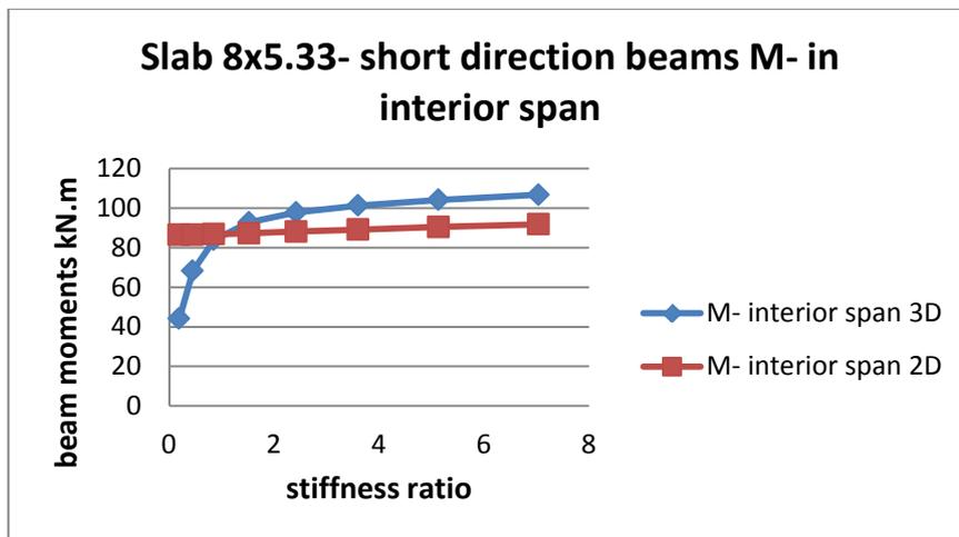
Figure 1 : Relation between moments in beams determined by three and two dimensional analyses- H
