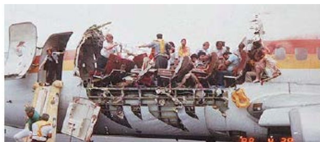
Figure 1 : Fuselage damage to Aloha Airlines Flight 243, April 1988
