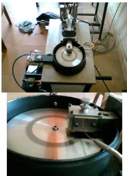
Figure 5 : Pin-on-disc wear tester
