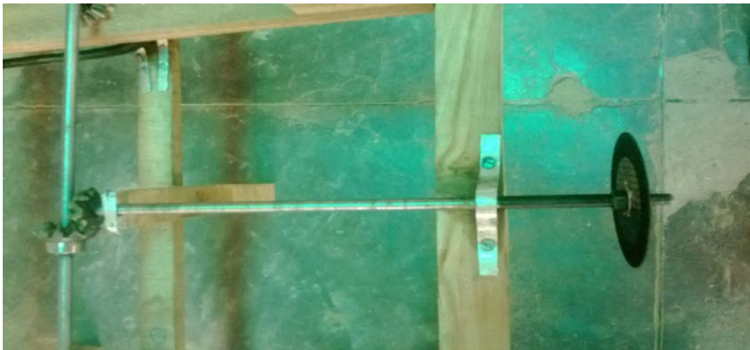
Figure 2 : Grinding Centre getting power through bevel gear arrangement
