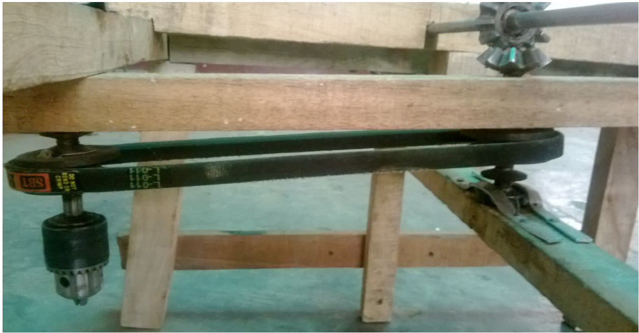
Figure 4 : Drilling centre getting drive through bevel gear and belt-pulley arrangement
