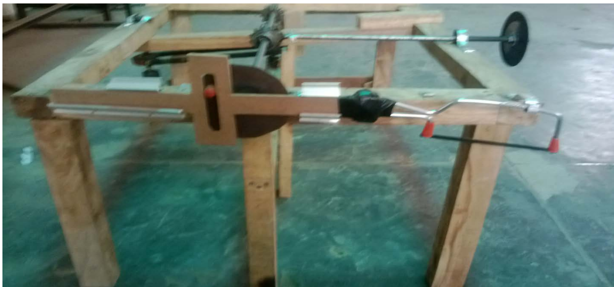
Figure 3 : Sawing/ Cutting end using Scotch Yoke Mechanism
