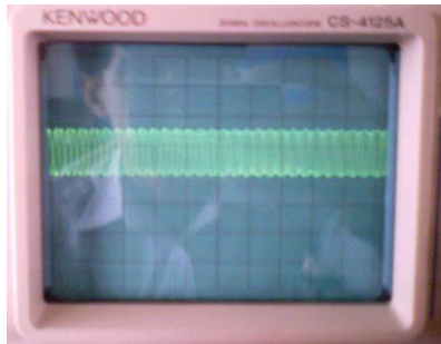
Figure 3 : Input signal fixed in 1.3 volt (pick to pick.)
