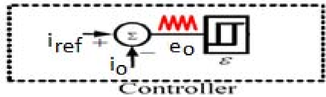
Figure 3 : Pictorial Representation of Error Current [8]
