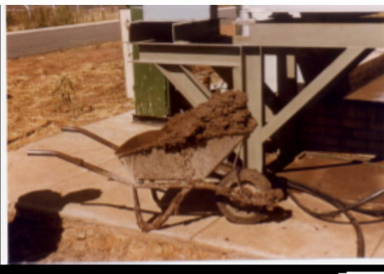
Figure 25: Centrifuge cake produced from HR clarifier sludge – cake dry solids 34.4% w/w, DOAA = 0,68 kg. (tss)-
