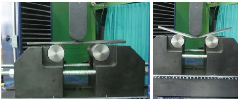
Figure 3: The Bending Test Process
