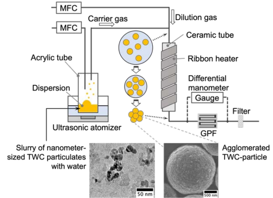
Fig. 3: Schematic diagram of the manufacturing process of TWC-particle membrane filter
