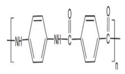
Aramid is the short component for aromatic polyamide. There are many brands of aramid fiber, but the wellknown one is Kevlar, and the others are Twaron, Technora, and SVM.
