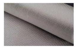
reinforcement of reinforced polymer composites due to their excellent electrical insulating properties, low susceptibility to moisture, and high mechanical properties.
