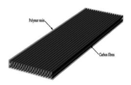
Carbon fiber has a high modulus of elasticity, 200-800 GPa. The final extension is 0.3 - 2.5%, where lower extension corresponds to higher hardness and vice versa.
