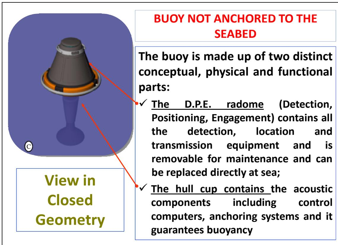
Figure 5: Image of the buoy not anchored in the "closed geometry"
