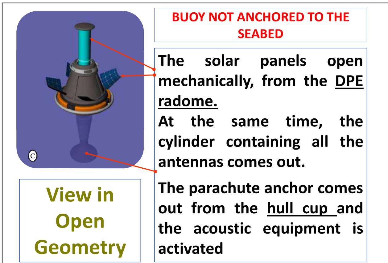
Figure 6: Image of the buoy not anchored in the "open geometry"
