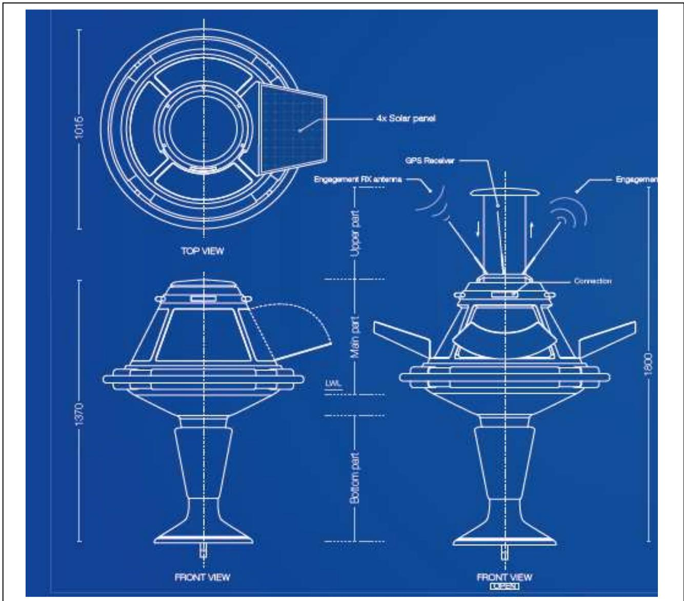
Figure 7: Dimensions of the buoy not anchored
