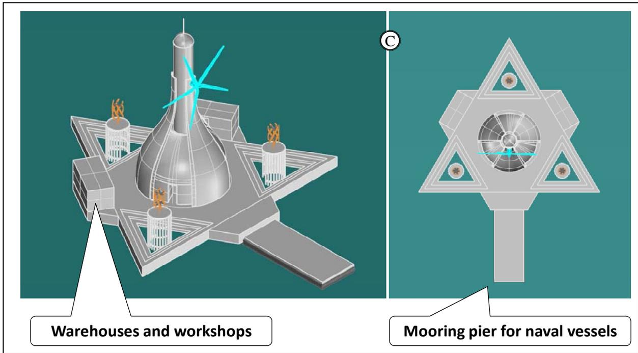
Figure 9: View of the wind platform where the docking capabilities of ships for refuelling or disembarking of personnel and warehouses/workshops are highlighted
