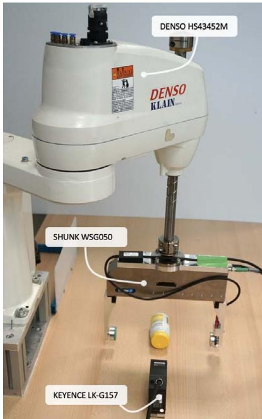
Fig. 6: System Architecture
