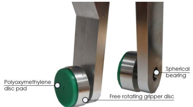
Fig. 1: Detail of the jaw provided of polymeric disc pad
