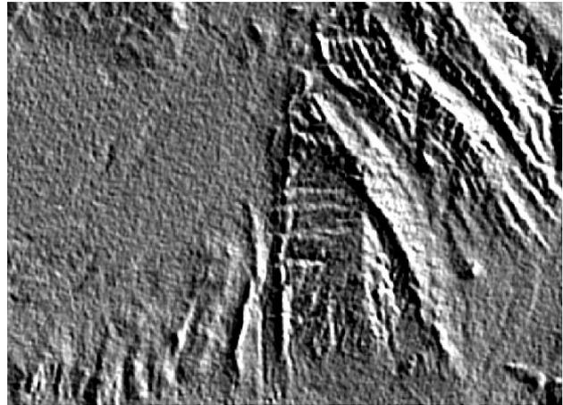
DEM in processing PCA algorithm by azimuths 0°; 45°; 90°; 135°; 180°; 225°; 270°; 315°
