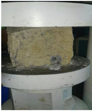
Fig. 8: Compressive Strength Test Failure Pattern on a Cube
