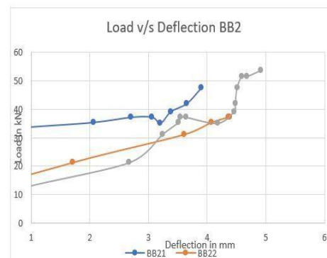
Fig. 13: Crack pattern as well as Basalt reinforced beam load-deflection graph
