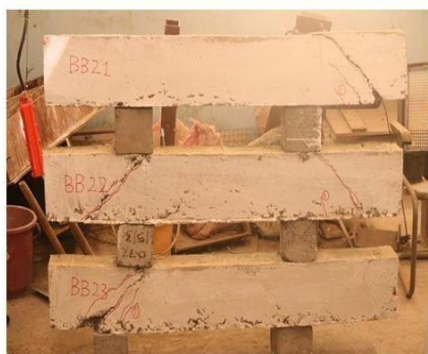
Fig. 13: Crack pattern as well as Basalt reinforced beam load-deflection graph
