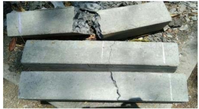
Fig. 9: For M20 grade concrete, prism failure patterns during flexural strength testing
