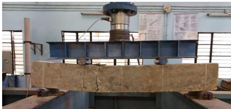
Fig. 4: Flexural Failure of beam
