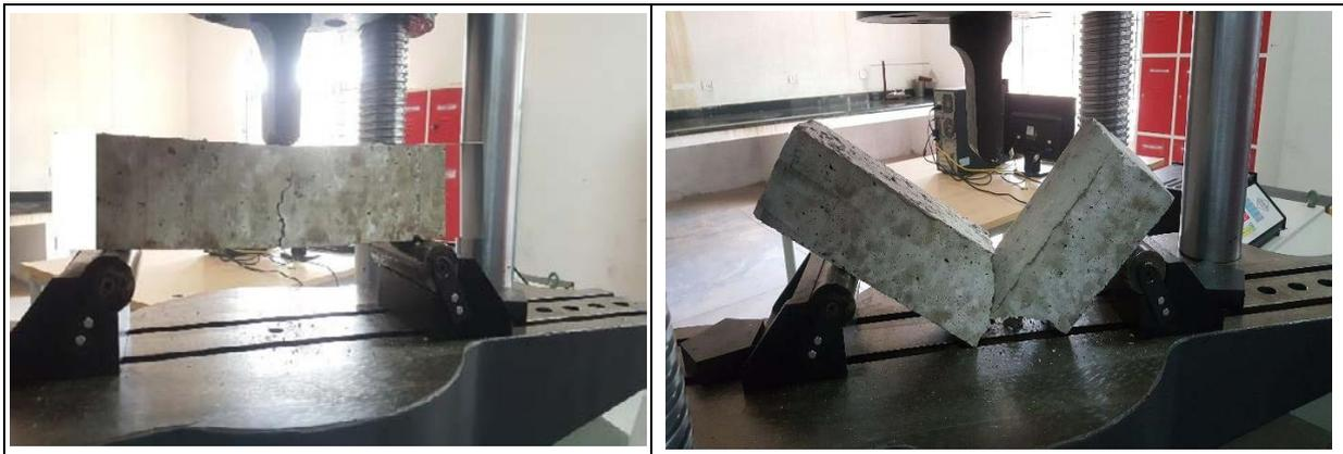
Figure 4: Single Point Load Testing on BFRGPC Specimen
