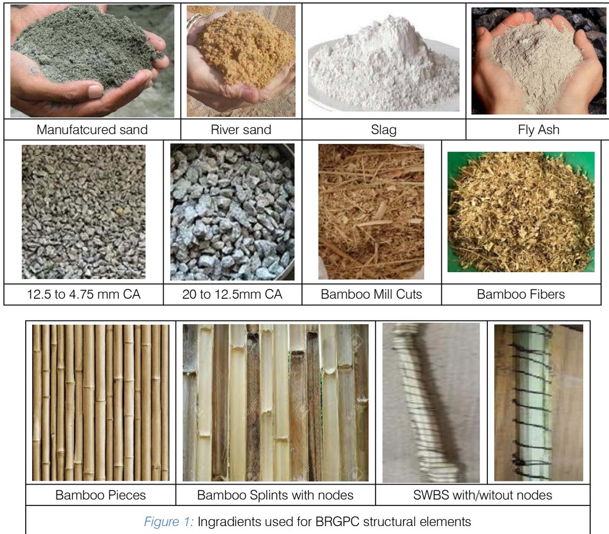
**Manufactured Sand:** Angular & rough texture need more water. Moisture is not held. Develops more strength compared to river sand. Silt content is zero. Granite compressive strength 100 to 250 Mpa and E = 20 to 70 GPa. M-Sand, crushed from granite stone, having Sp.gr 2.45, Fineness Modulus (F.M) 2.70.
