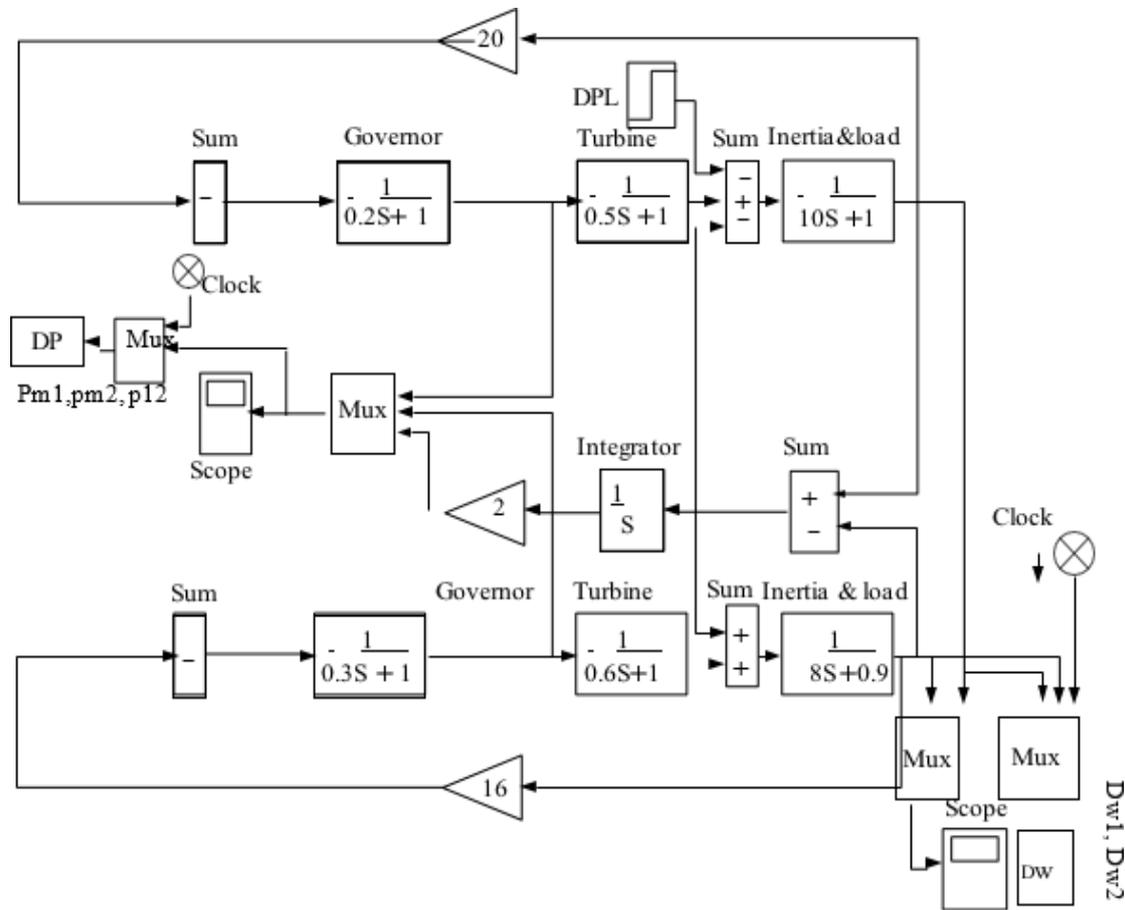
Figure 1: Model of two areas load frequency control
