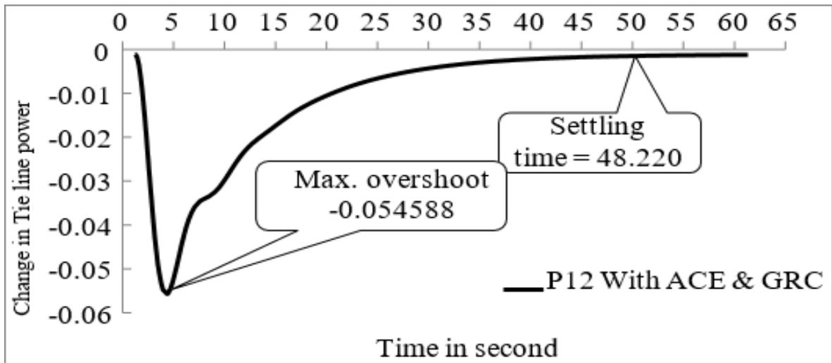
Figure 14: Change in tie-line power of two areas with ACE and GRC
