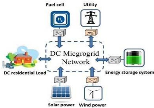
Fig. 1: Schematic of a conventional microgrid system
