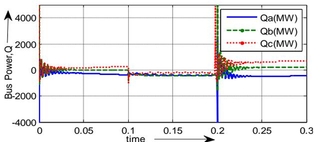
Figure 16 : Bus Power, Q for 1-∅ fault in MW (with POC)
