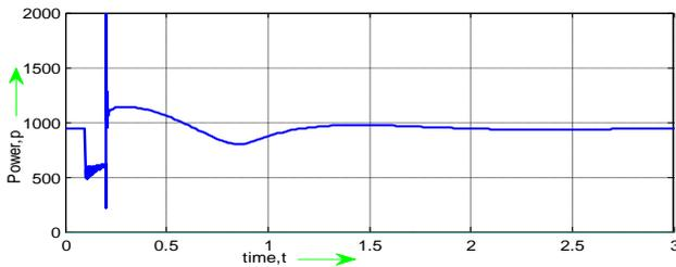
Figure 6 : Bus Power (P) in MW for 1-Ø faults (with STATCOM)
