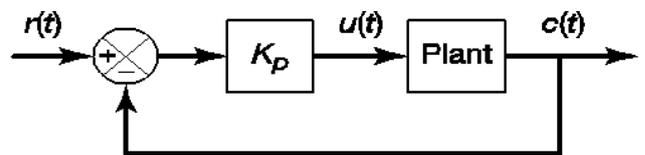
Figure 8 : PID controller is in proportional action
