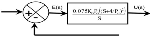
Figure 10 : PID controller with tuning parameters
