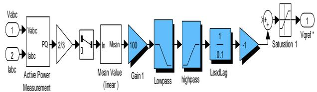
Figure 12 : Internal Structure of POD controller
