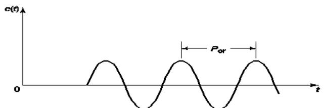
Figure 9 : Determination of sustained oscillation (Pcr)
