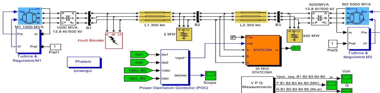
Figure 2 : Complete simulink model of 2-machine power system
