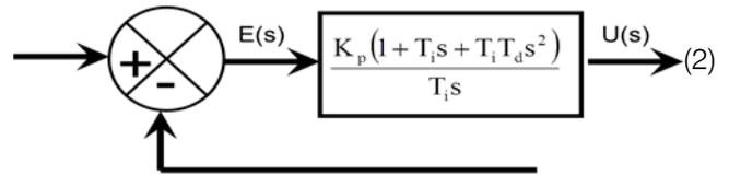
Figure 7 : Block diagram of PID controller parameters
