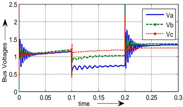
Figure 15 : Bus voltage in p.u for 1-∅ fault (with POC)
