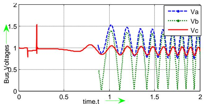
Figure 3 : Bus voltages for 1-phase fault (without STATCOM)
