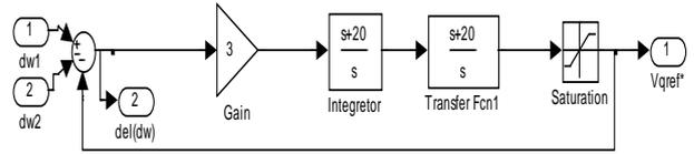
Figure 11 : Internal Structure of PID Controller
