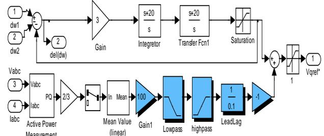
Figure 13 : Internal Structure of Power Oscillation Controller (POC)
