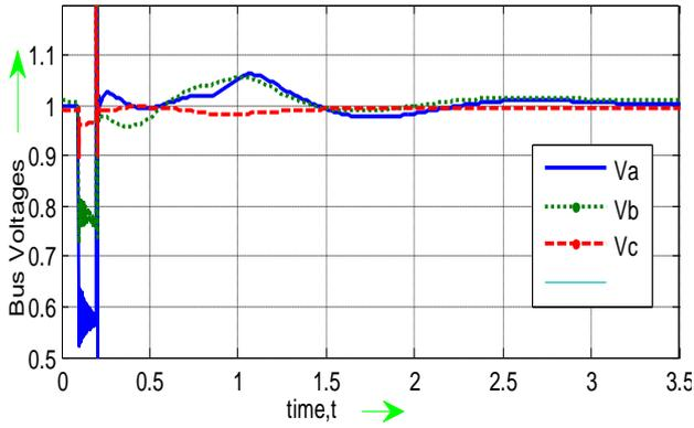
Figure 4 : Bus Voltages in p.u for 1-phase fault (with STATCOM)
