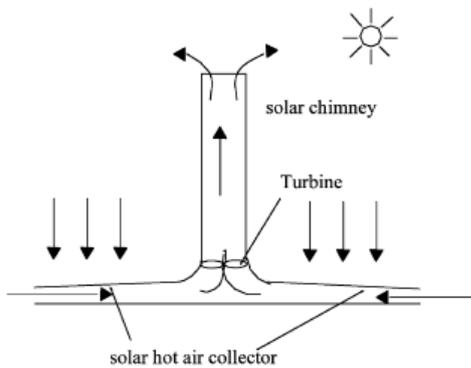
Fig. 1 : Schematic diagram of a solar power plant
