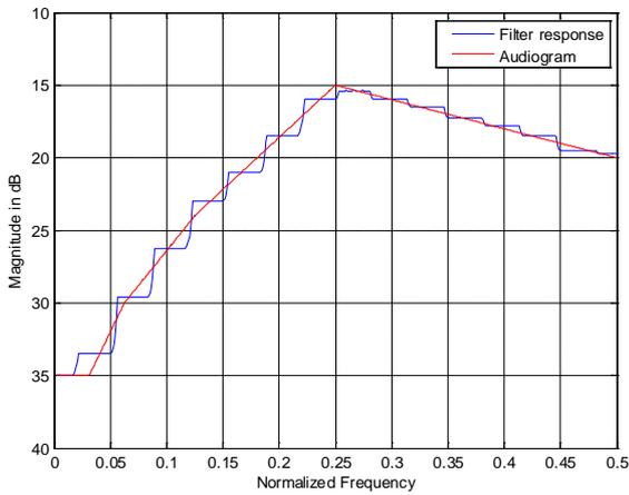
Figure 9 : Audiogram fitting for the uniform filter bank
