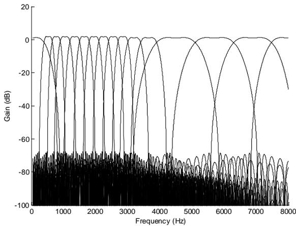
Figure 7 : Frequency response of the uniform filter bank derivatives at the offset position  $k/M$  from the interpolating output phase centre. The computed output is formed from a local Taylor series as given by Equation (1).
