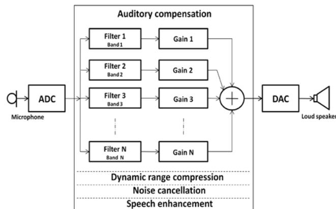
Figure 1 : Block diagram of digital hearing aid
