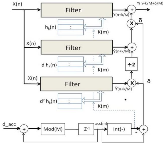
Figure 6 : Implementation of arbitrary sample rate converter
