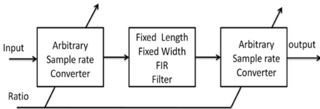
Figure 5 : Functional block diagram of variable bandwidth filter
