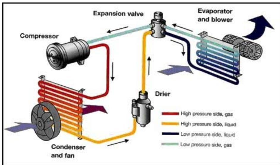
Fig. 2 : Existing Refrigeration system in automobiles
