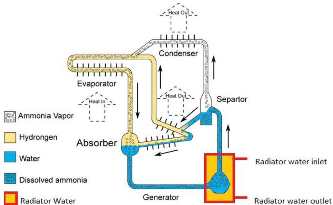
Fig.3 : Schematic of a triple fluid vapours absorption refrigeration system
