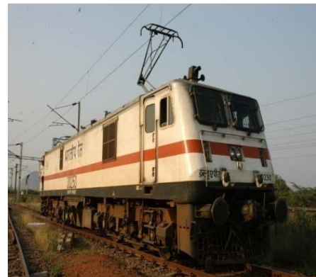
Fig.1 : Electric Locomotive with panto raised condition.
