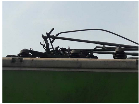
Fig. 5 : Electric Locomotive with Broken Pantograph
